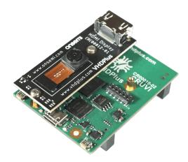
Despite so many components, the system is only  $5.6 \times 4.5 \times 2.2$  cm in size. It is ideal for testing the performance of FPGAs in image processing, and the AR0430 camera offers much more capability than used here. But with the CURVI connector the camera can also be connected to faster FPGAs to use the full potential.
